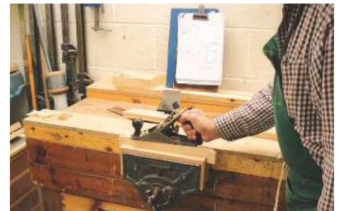
▲ Pic.9 Remove the tongue from the back edge and plane off the last of the tongue...
